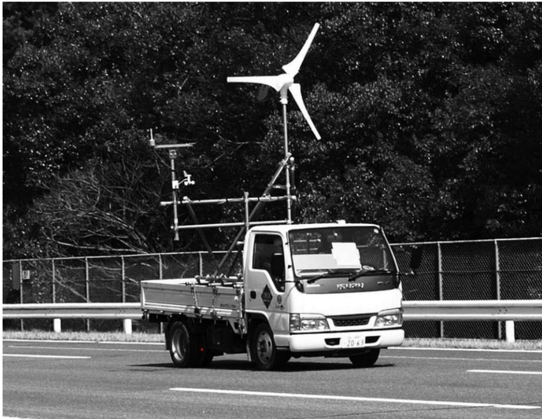
Figure 2.12: On-road performance assessment of a wind turbine mounted on a mobile vehicle-based testing rig (Adapted from Matsumiya et al., 2010).
