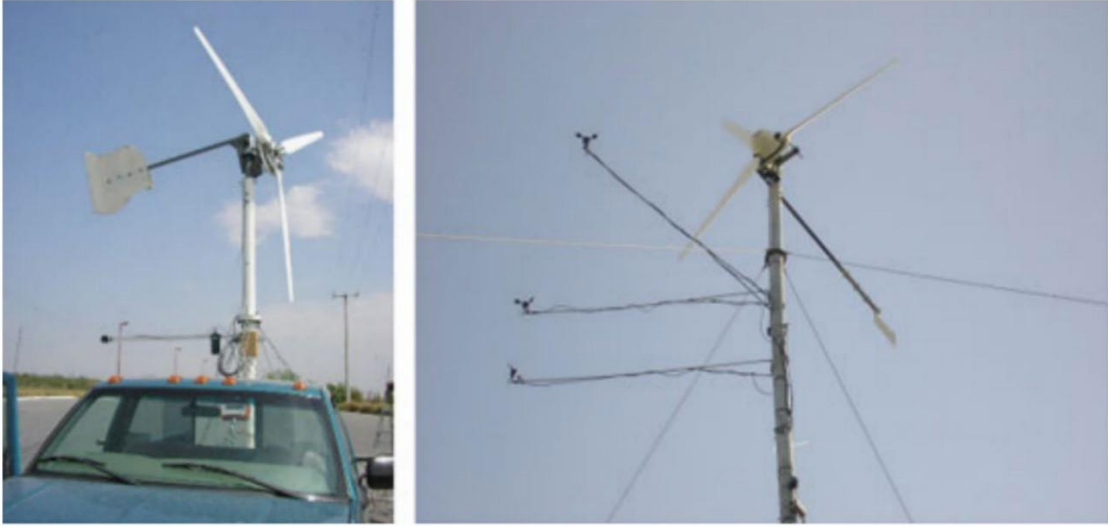
Figure 2.6: Experimental configuration for Aeroluz wind turbine testing, illustrating (a) a mobile truck-mounted system and (b) a fixed field installation. (Adapted from Elizondo et al., 2016)
