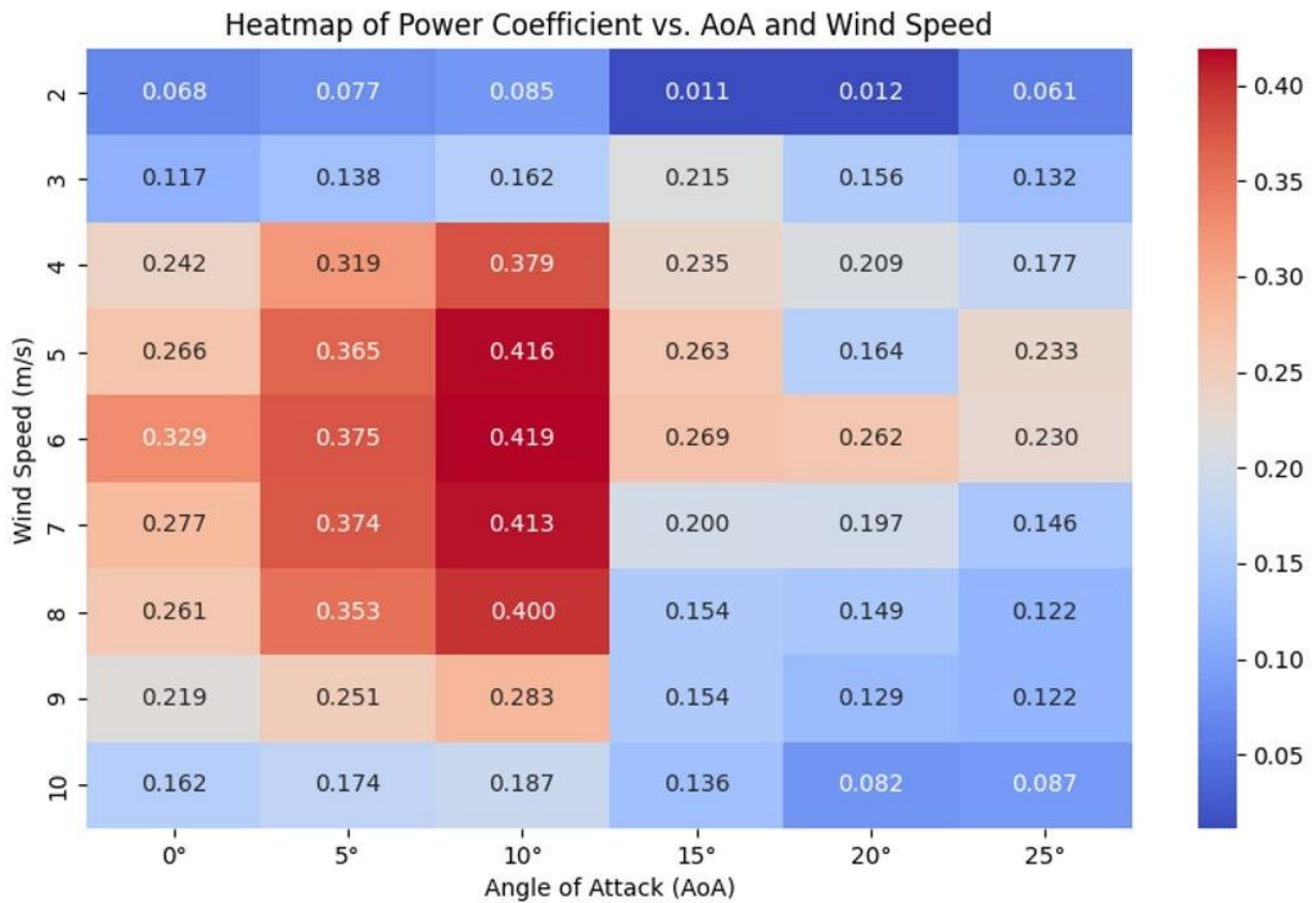
Figure 4.4: Heatmap of power coefficient ( C_p ) across wind speeds and angles of attack
