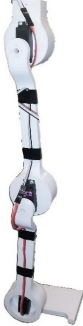
Figure 5.3 Leg of the LLE prototype made of PLA in white colour
