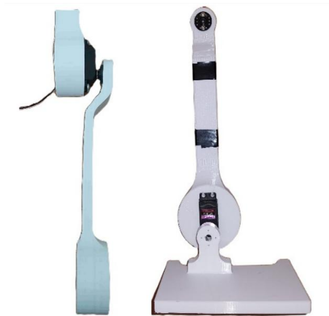
Figure 5.11: Right to left, the thigh connects to the hip, and the shank to the foot.
