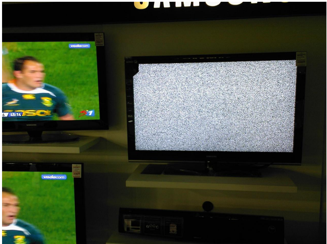
Figure 4.14: Television set to display snow pattern for testing (Bredekamp AJ, 2010)
