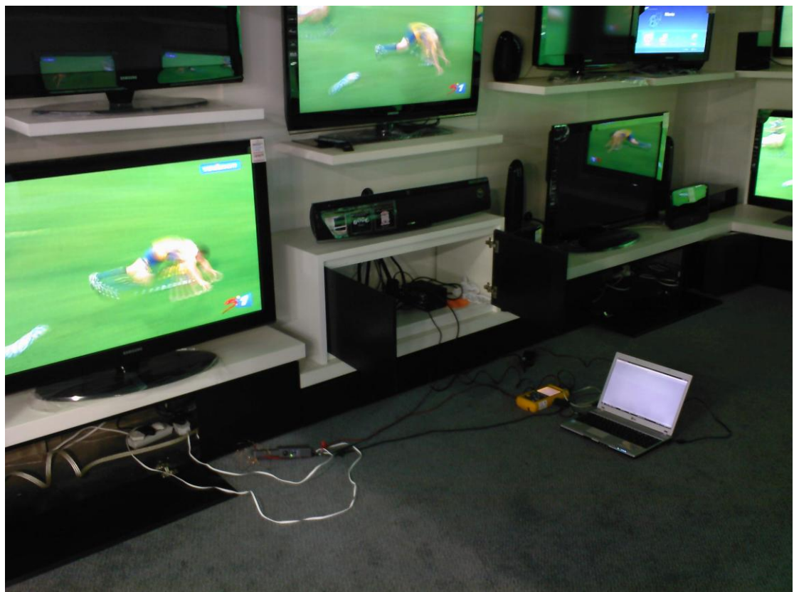
Figure 4.15: The power consumption of a television set being measured showing the current clamp arrangement, Fluke 43B and laptop computer (Bredekamp AJ, 2010)
