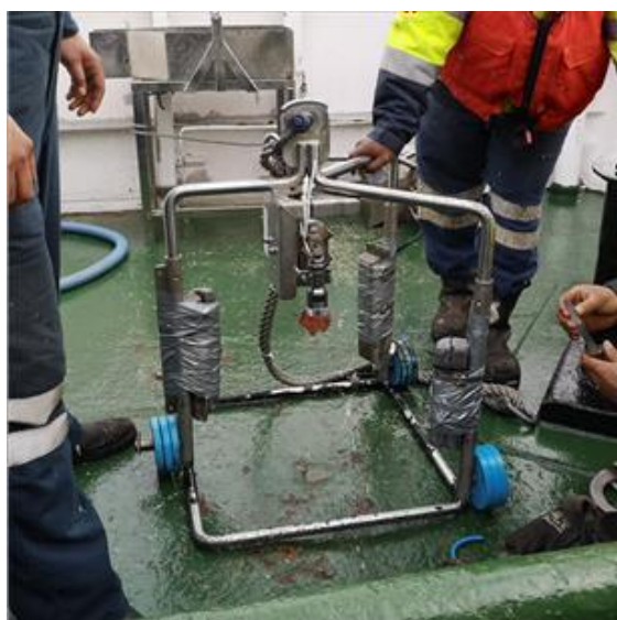
Appendix 4.1. Weights added and secured to the Drop camera system
