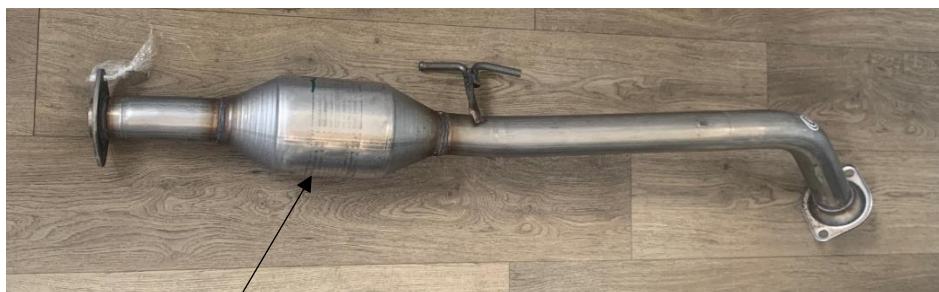
Figure 5 Catalytic converter before dismantling (the ceramic catalyst is contained in the part shown by the arrow)
