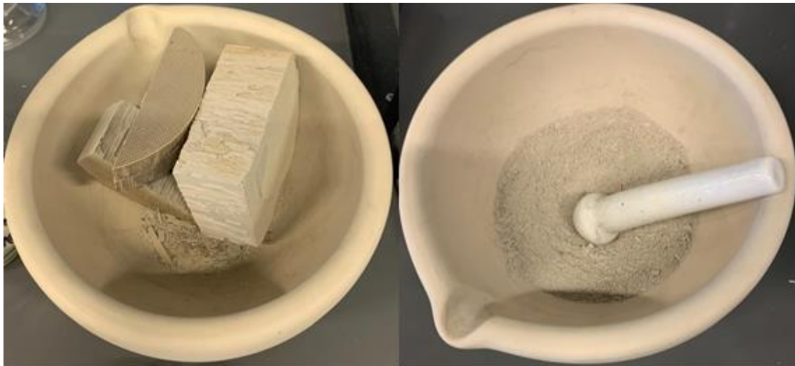
Figure 9 Size reduction using a pestle and mortar
