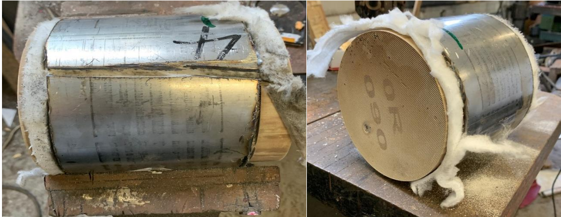
Figure 7 Catalytic converter before final steel housing removal
