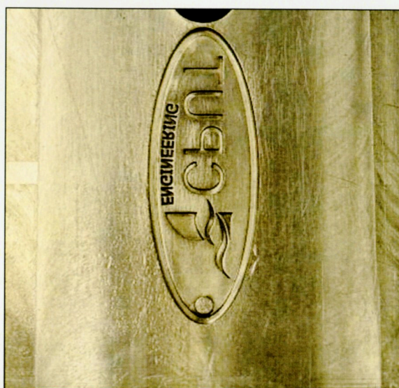
Figure 5.15: Aluminium injection side insert after moulding. Note the pitting marks
