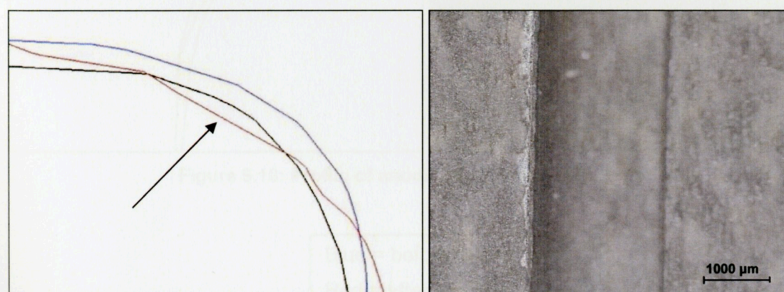
Figure 5.7: Profile of anodised, injection side lower logo edge (irregular profile produced after moulding with some material loss)
