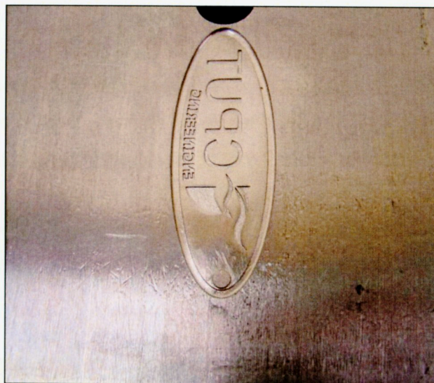
Figure 5.14: Steel injection side insert after moulding. Note the pitting marks
