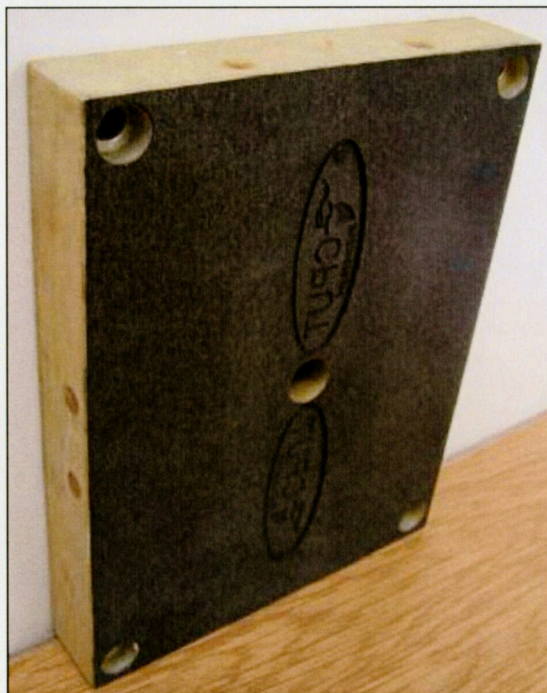
Figure 4.20: AA7075 injection side insert after hard anodising. Note the lacquer around the edges and holes
