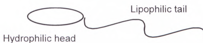
Figure 2.8: Schematic structure of surfactant molecule
