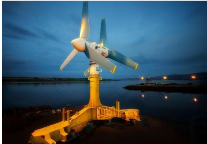
Figure 25. The in-stream tidal turbine known as AR1500, which is anchored to the seabed, originates from SIMEC Atlantis [109].
