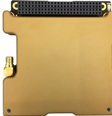
Figure 2.2: Cubesat SDR-based AIS Receiver ( BR-01-00150 Rev A, CPUT, 2022)
