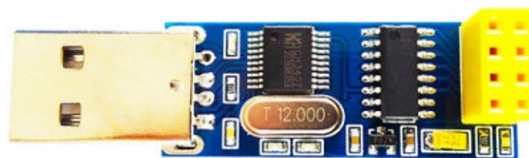
Figure 3.6: USB Adapter for NRF24L01+ (USB Adapter for NRF24L01+, 2022)
