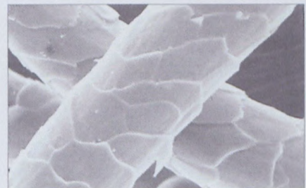
Figure 4.2. Image of magnified barbed wool fibre. White. 2007: 9.
