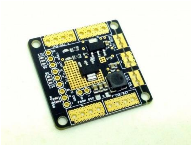
Figure 2.11: Power Distribution Board
