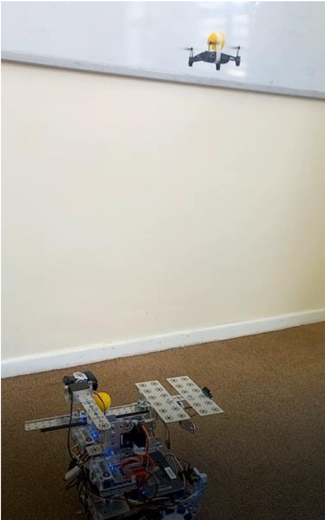
Figure 4.3: Docking system just after take-off Note that the docking arm retracts back to its initial position
