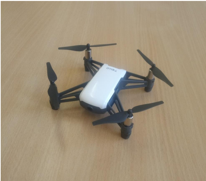
Figure 3.8: DJI tello drone without propeller guards Propeller guards were taken off to reduce the instability while hovering at low heights due to ground effect.
