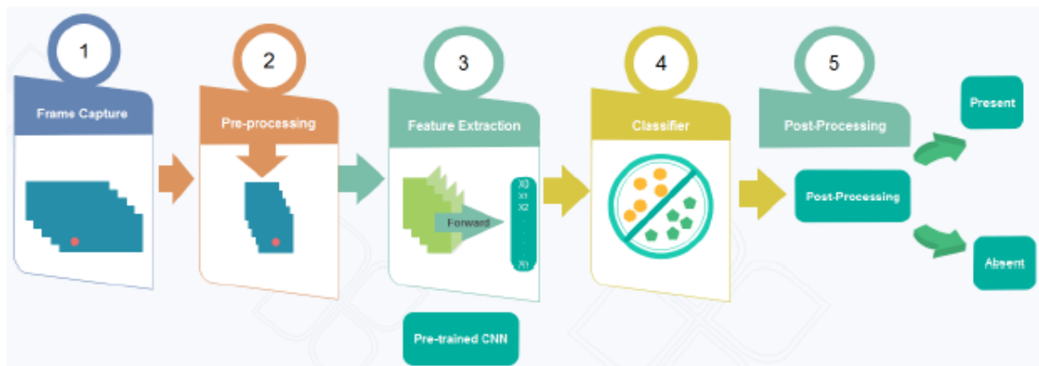
Figure 2.21: Block Diagram of SAR System Using UAVs with Machine Learning Technology (Adapted from (Hazim, et al., 2019))
