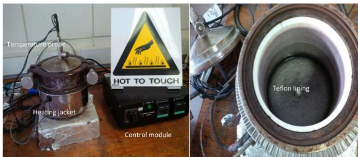
Figure 3.2: Reactor setup for preparation of \beta -FeOOH
