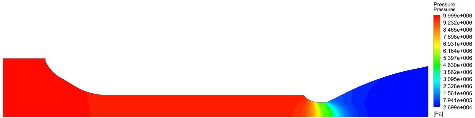
Figure F.14: Case 2-1 - Iso pressures
