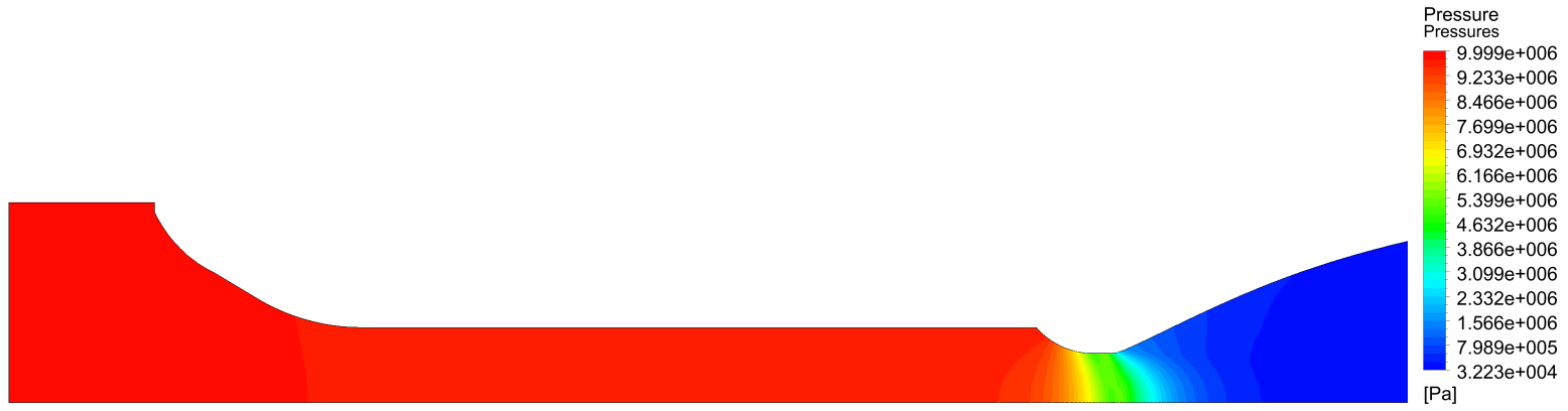
Figure F.24: Case 2-3 - Iso pressures
