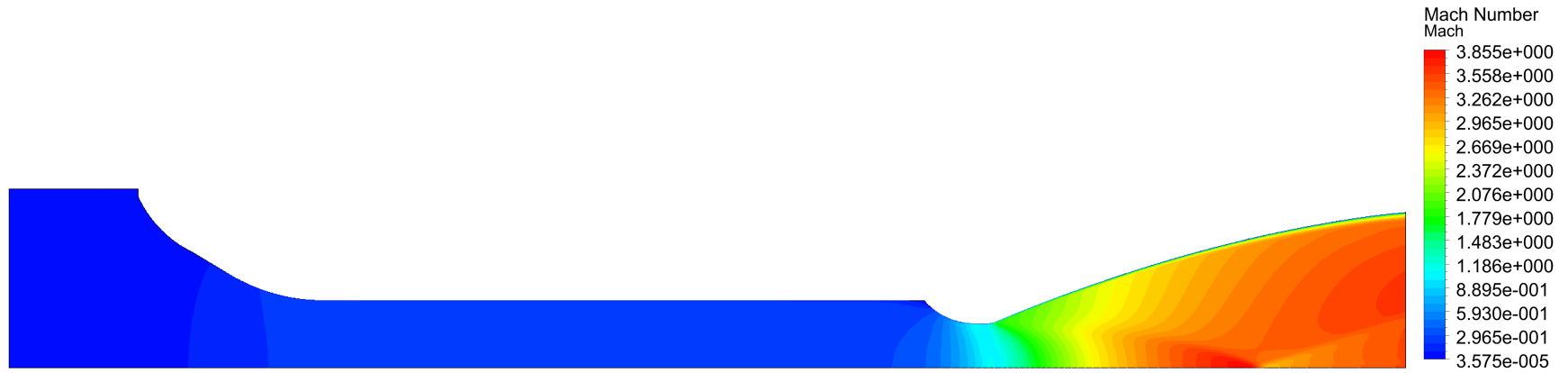
Figure K.18: Case 5 - Full length Rao parabolic approximation - Iso Mach numbers
