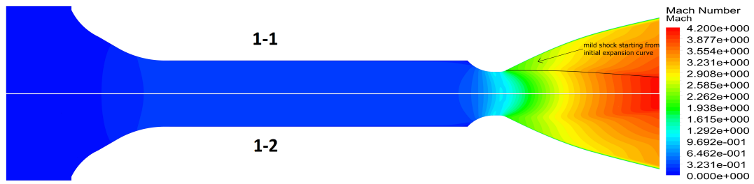
Figure 5.13: Mach number comparison of 1 – 1 and 1 – 2
