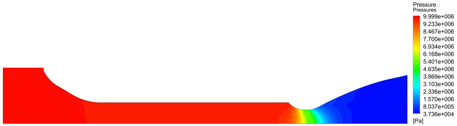
Figure F.29: Case 2-4 - Iso pressures
