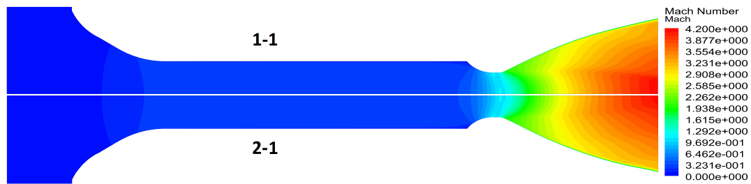
Figure 5.19: Mach number comparison of 1 – 1 and 2 – 1
