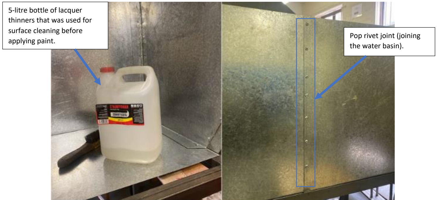
Figure 3.2: Water basin construction
