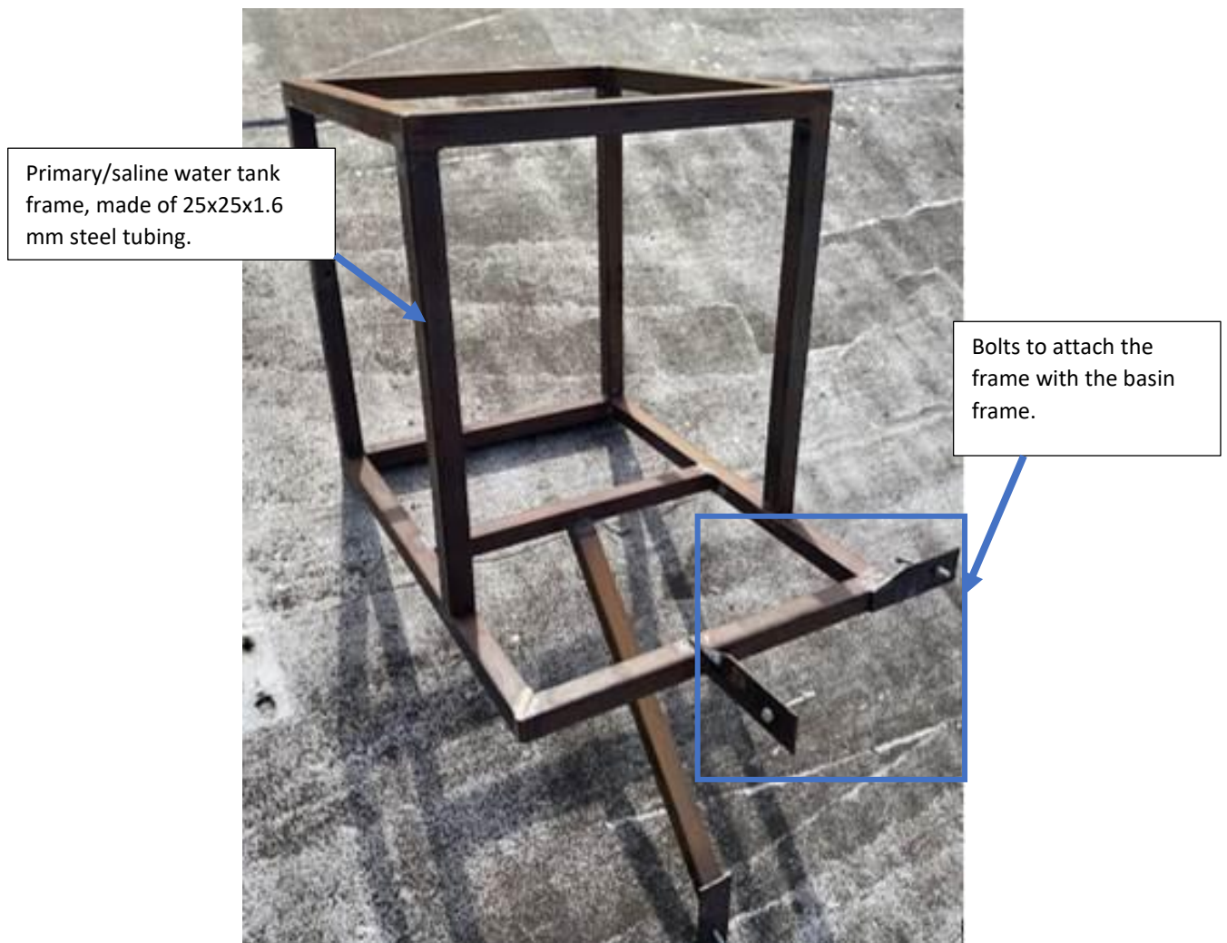
Figure 3.13: Saline water tank frame (before painting)
