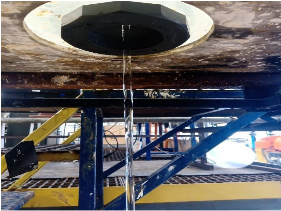
Figure 3.8: Orifice attached to the base center of the tank discharging glycerine solution
