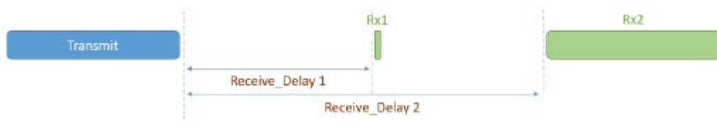
Figure 2.7: Received window: Rx 2 window received packet
