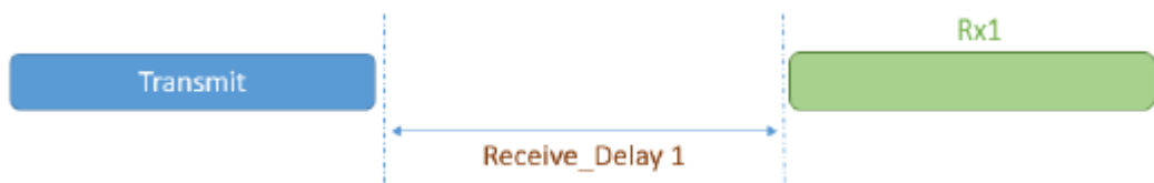
Figure 2.6: Received window: Rx 1 window received packet
