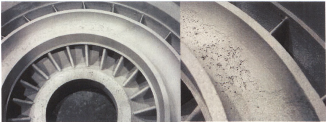
Figure 5.9 Porosity shown in Casting
