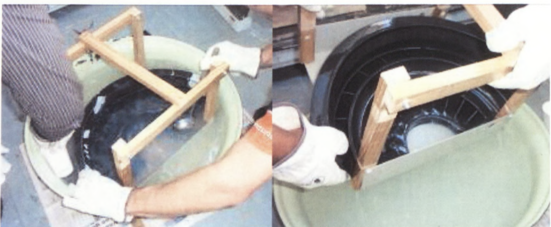
Figure 5.3 Wax Infiltration of Pattern
