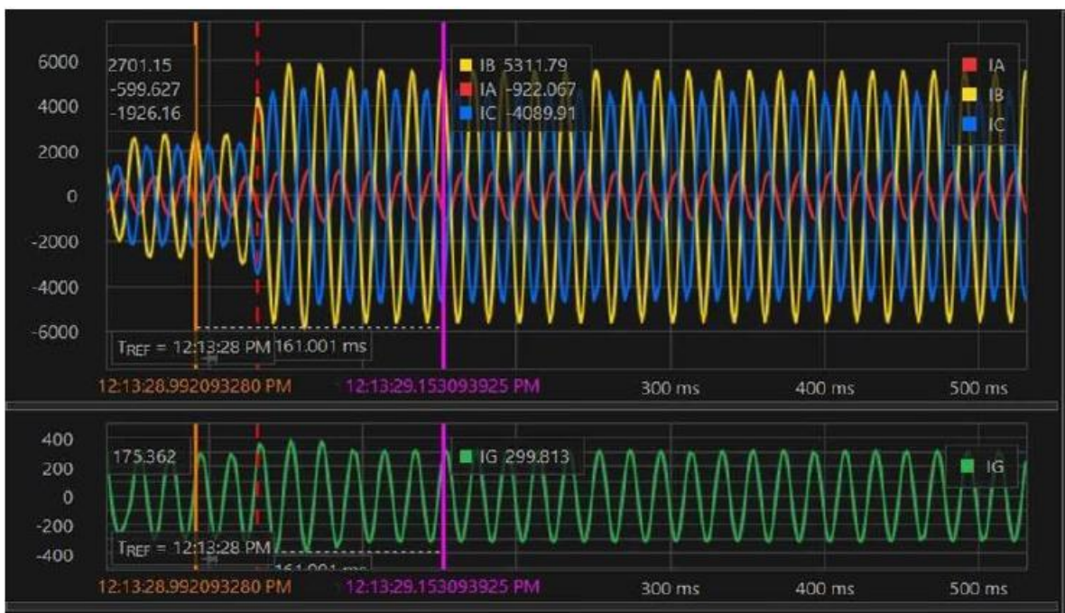
Figure 5.3: Transformer fault current
