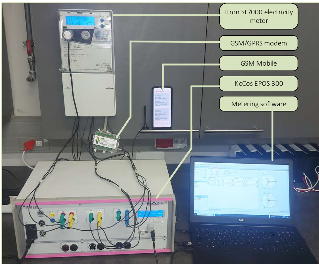
Figure 4.2: Test setup in laboratory
