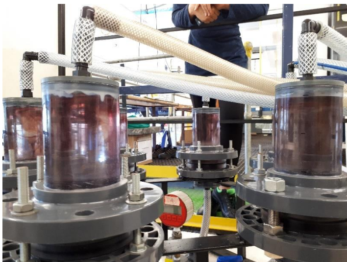
Figure C.6: Reactor columns with degraded real effluent at 70 minutes of running time
