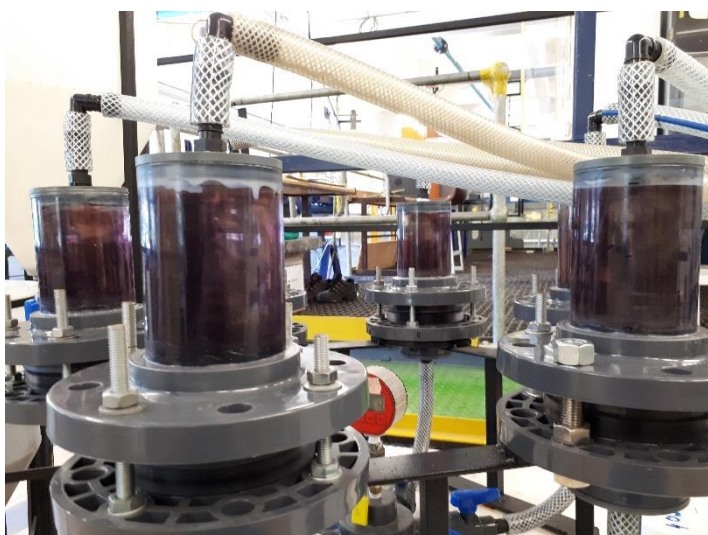
Figure C.4 Reactor columns with degraded real effluent at 40 minutes of running time
