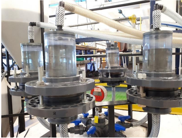
Figure C.1: Reactor columns with degraded real effluent at 2 minutes of running time
