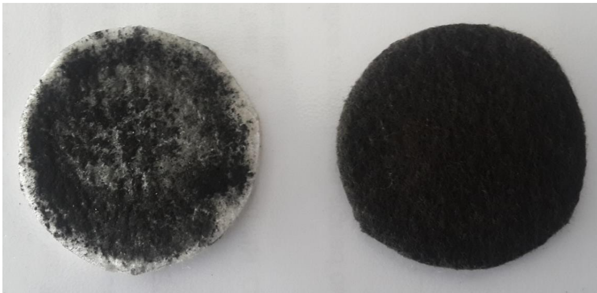
Figure 3.8: Reaction barriers with catalyst being immobilized by two different techniques; hand spread catalyst technique (left) and the Buchner filtration method (right)
