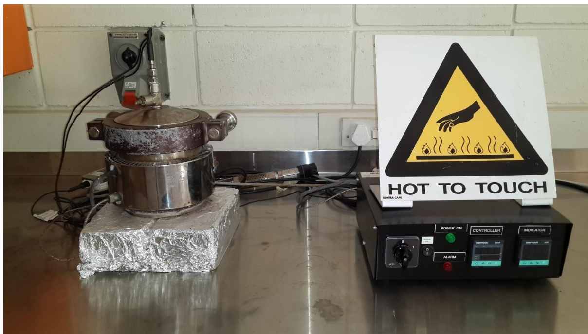
Figure 3.1: One litre Teflon-lined autoclave used to synthesize the batch \text{Co}_3\text{O}_4
