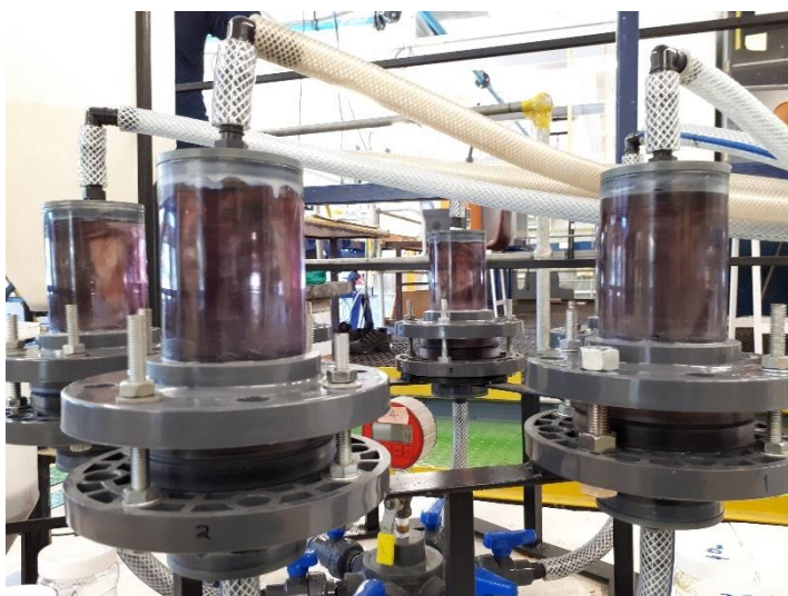
Figure C.5: Reactor columns with degraded real effluent at 60 minutes of running time
