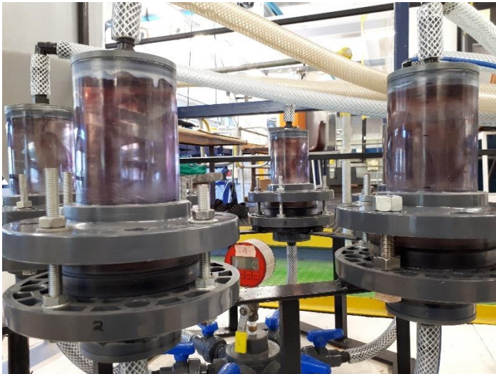
Figure C.2: Reactor columns with degraded real effluent at 20 minutes of running time
