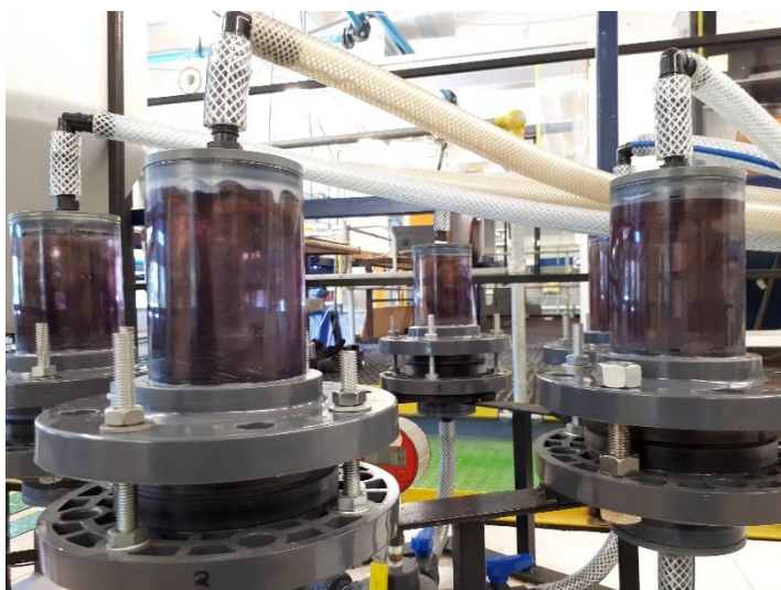
Figure C.3: Reactor columns with degraded real effluent at 30 minutes of running time
