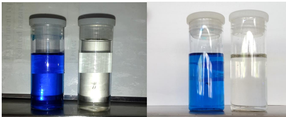
Figure 3.20: Feed and product samples for the degradation of methylene blue prepared by using de-ionised water (left) and tap water (right)
