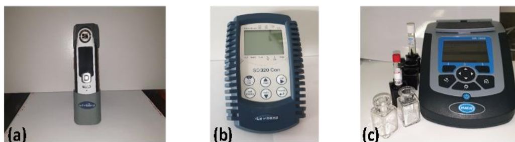
Figure 3-11: (a) Lovibond colourimeter, (b) Lovibond SD 320 Conductivity waterproof Handheld meter and (c) DR1900 spectrophotometer
