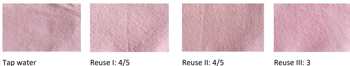
Figure 4-15: Colour fastness of the dyed fabrics after 48 hours of standing time of the treated effluent before reuse
