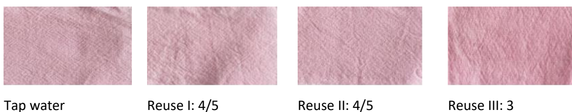
Figure 4-14: Colour fastness of the dyed fabrics after 5 hours standing time of the treated effluent before reuse
