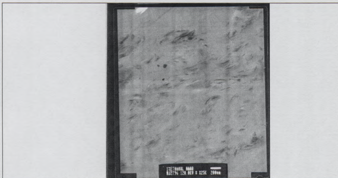
Figure 5.9: A TEM image of 1% hydroxyethylMMT-PS nanocomposite magnified at 200nm scale.
