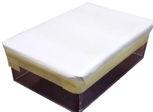
Photo 3-2: Rectangular frame with membrane fixed for modification
