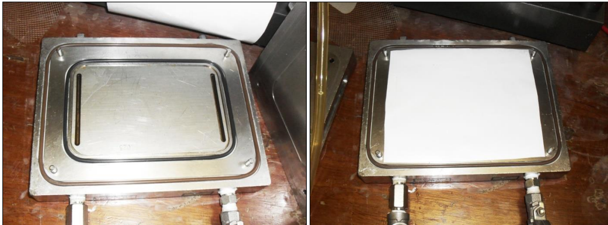
Photo 3-14: Pictures illustrating the position of sealers on the module (left) and the correct placement of membrane on module (right) (lab 1.1, science building, CPUT, August 2017)
