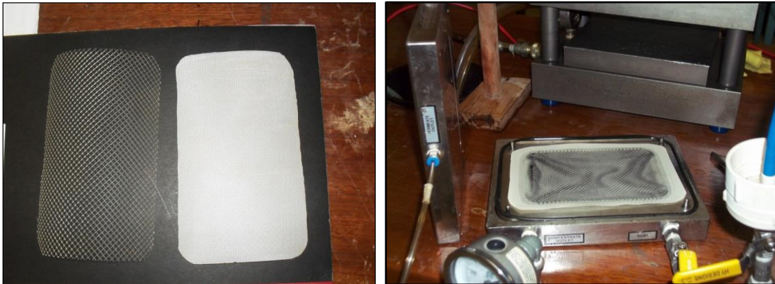
Photo 3-13: Pictures showing the two different spacers (left) and membrane placed with spacers in the cell (right) (lab 1.1, science building, CPUT, August 2017)
