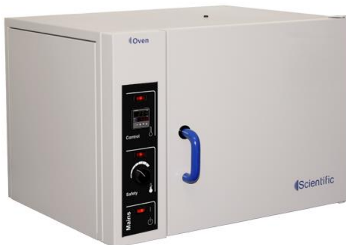
Photo 3-4: Oven model used during modifications of membranes
