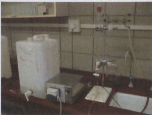
Figure 2.1: Regeneration of resin
