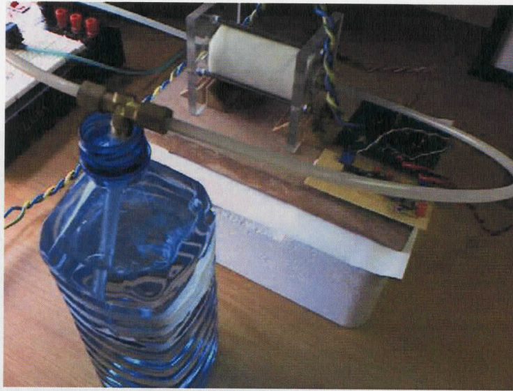
Figure 8-4: A compressor in action, shown by pumping compressed air through water in a bottle
