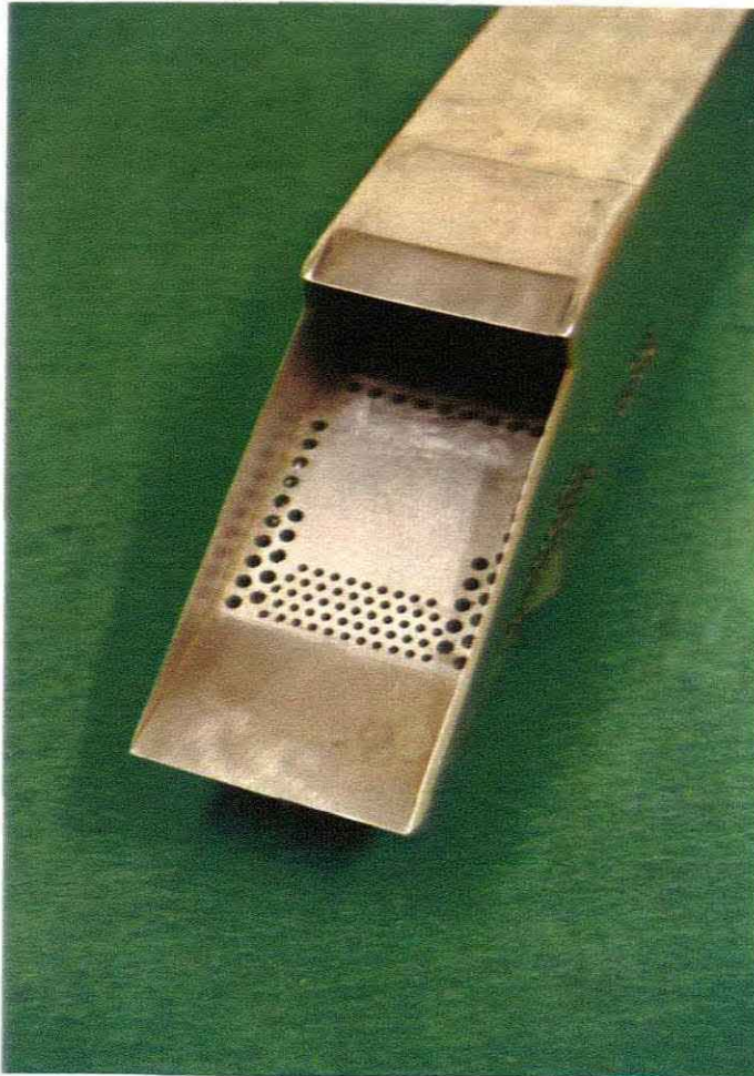
FIGURE 4.7 : Frontal View of Model Showing Bleed Holes
