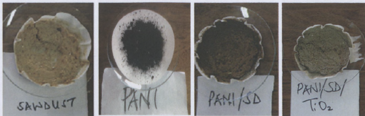
Figure 4.2: Images of SD, PANI, PANI/SD and PANI/SD/TiO 2 after synthesis.
