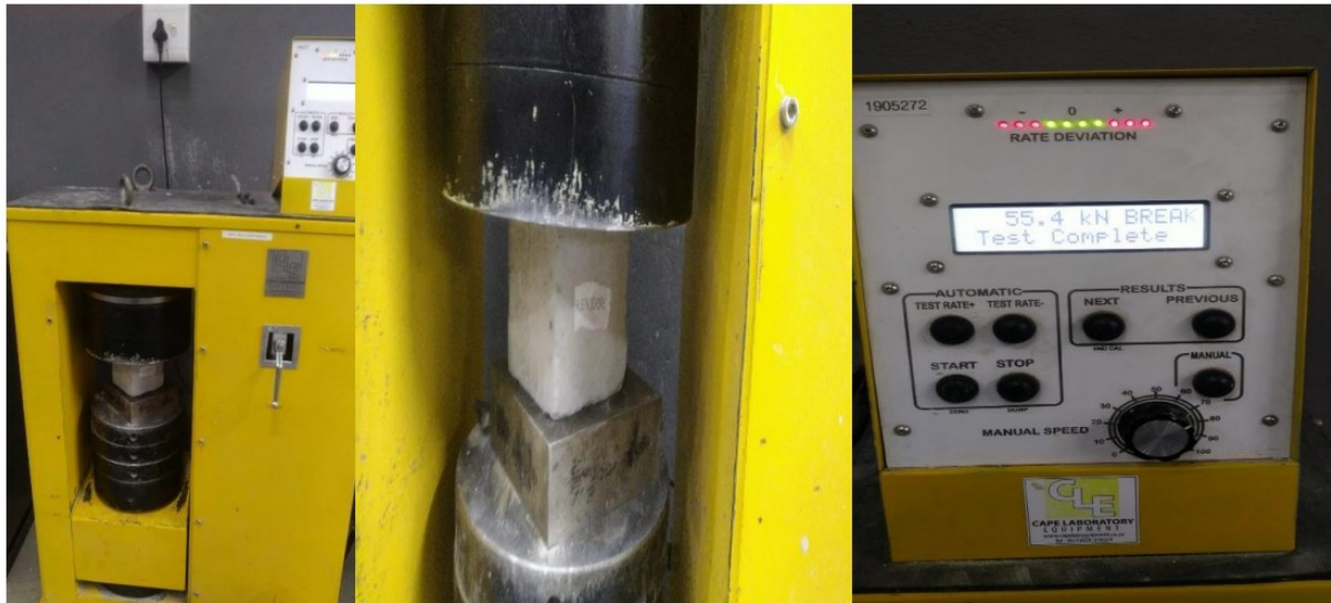
Figure 3.9: Specimen testing for compressive strength.
