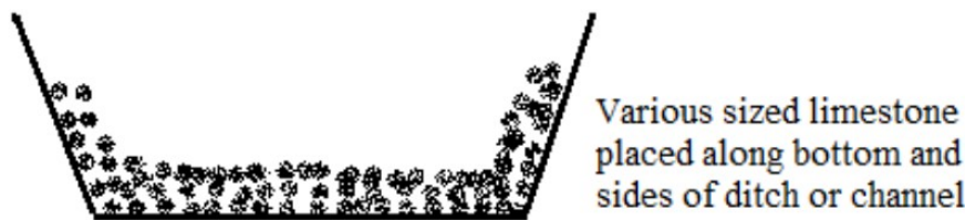
Figure 2.13: Cross section of an open limestone channel (Seervi et al., 2017).
