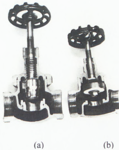
Figure 2.9: Internal structure of globe valves: (a) with plug (b) with composition disc
