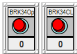
Figure 7.12: Pushbuttons used to open and close circuit breakers during runtime
