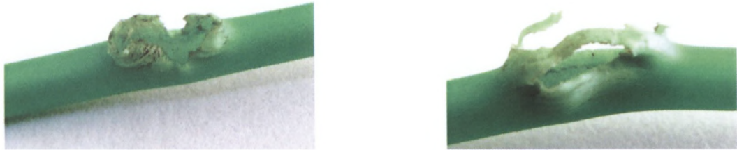
Figure 3.13: Pictures of typical bursts observed during burst strength test
