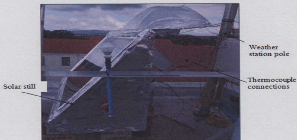
Figure 3-7: Perspective view of the test rig on roof top
