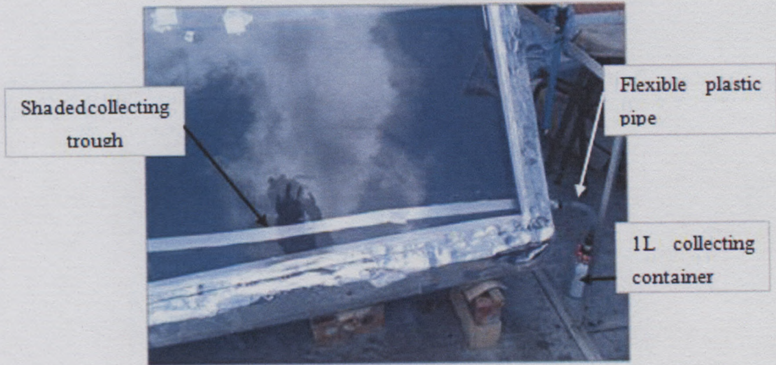
Figure 2-7: Front cover collecting system
