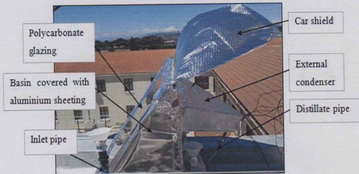
Figure 2-9: Side view of the still
