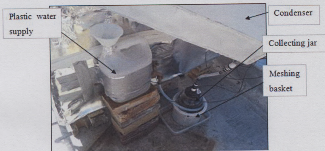
Figure 2-10: Evaporative cooling system
