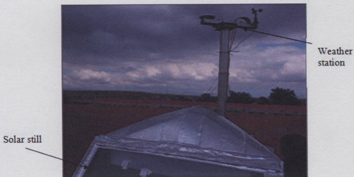
Figure 3-7: Perspective view of the test rig on roof top
