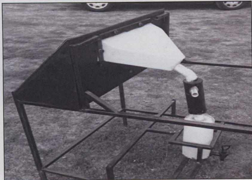
Figure 2-11: Solar still model
