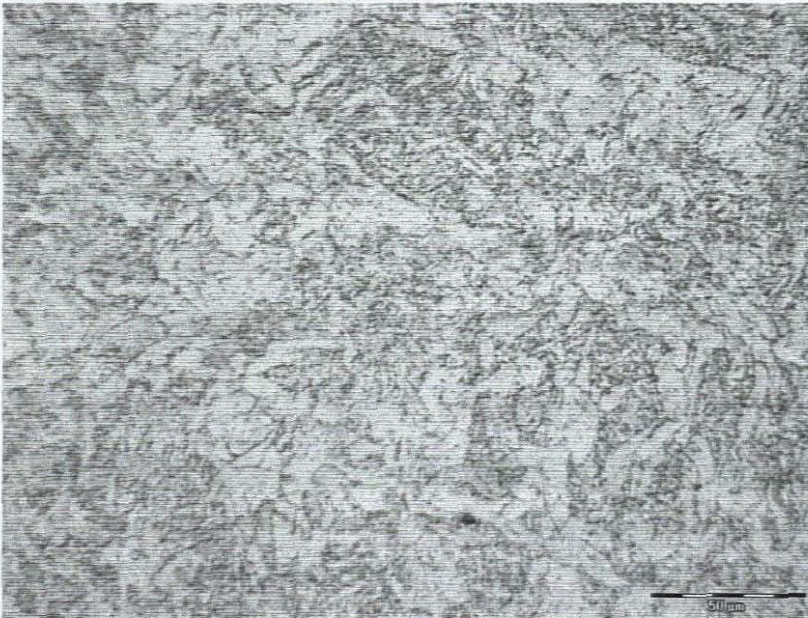
Figure 7.65 Microstructure of weld specimen 4 depicts a structure of acicular ferrite (Widmanstätten) with pearlite as seen at 50\mu\text{m} = 20\text{mm} \Rightarrow 400\times .
