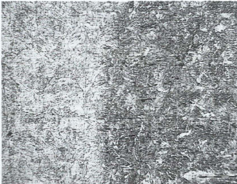
Figure 7.70: Microstructure of weld (RHS) and the HAZ (LHS) of specimen 5. The weld displays ferrite grains in a pearlite matrix as seen at 100\mu\text{m} = 16.75\text{mm} \Rightarrow 167.5\times .
