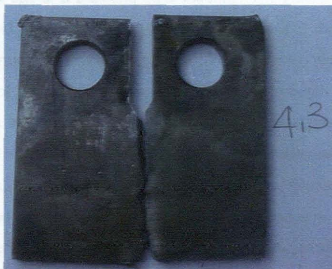
Figure 7.23: Specimen 4.3 depicts a fracture through the centre of the weld.
