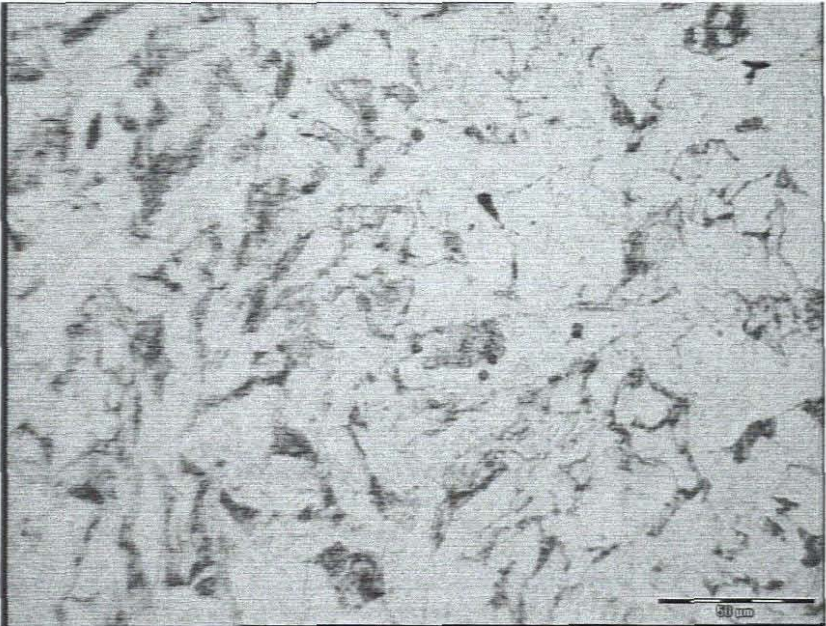
Figure 7.45 Microstructure of the HAZ specimen 3 depicts a structure of equiaxed ferrite grains with pearlite islands as seen at 50μm = 20mm ⇒ 400x.
