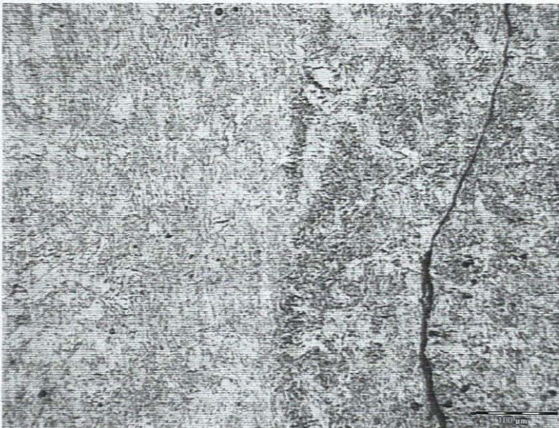
Figure 7.61: Microstructure of specimen 2 clearly depicting a difference in microstructure between the weld (RHS) and the HAZ (LHS). Note the crack in the weld area as seen at 100\mu\text{m} = 16.75\text{mm} \Rightarrow 167.5\times .
