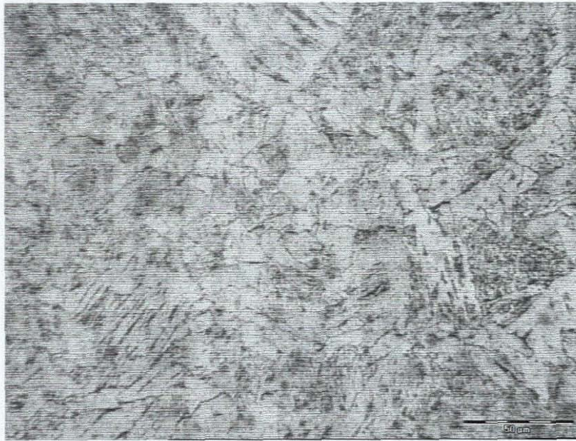
Figure 7.68: Microstructure of the weld specimen 5 depicts a structure of acicular ferrite (Widmanstätten) with pearlite as seen at 50\mu\text{m} = 20\text{mm} \Rightarrow 400\times .
