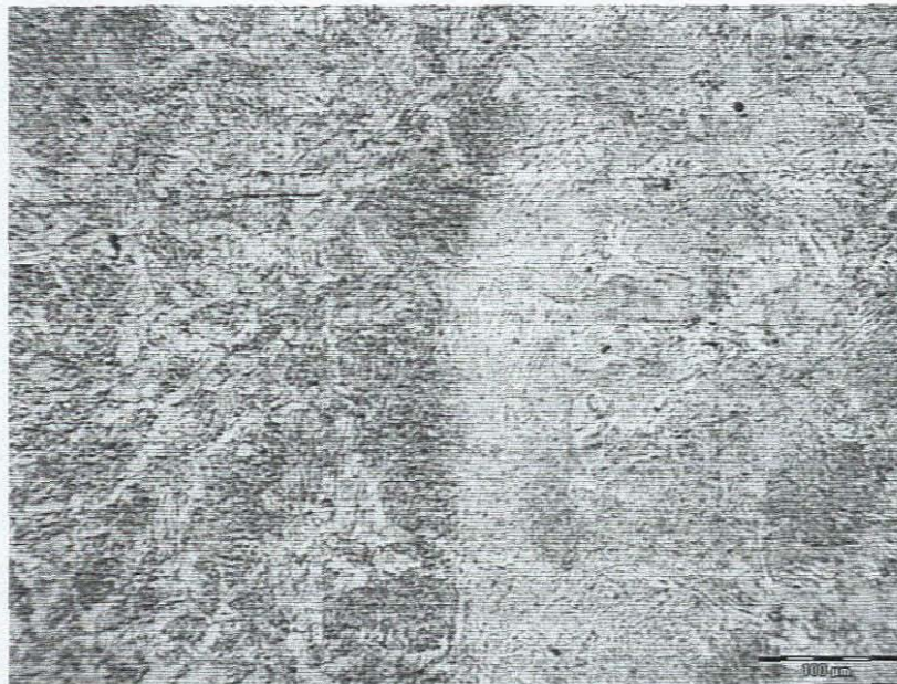
Figure 7.67: Microstructure of weld (LHS) and the HAZ (RHS) of specimen 4 with a distinct difference in the microstructures as seen at 100\mu\text{m} = 16.75\text{mm} \Rightarrow 167.5\times .
