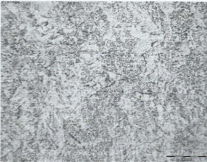
Figure 7.59: Microstructure of weld specimen 2 depicts a structure of acicular ferrite (Widmanstätten) with pearlite as seen at 50\mu\text{m} = 20\text{mm} \Rightarrow 400\times .
