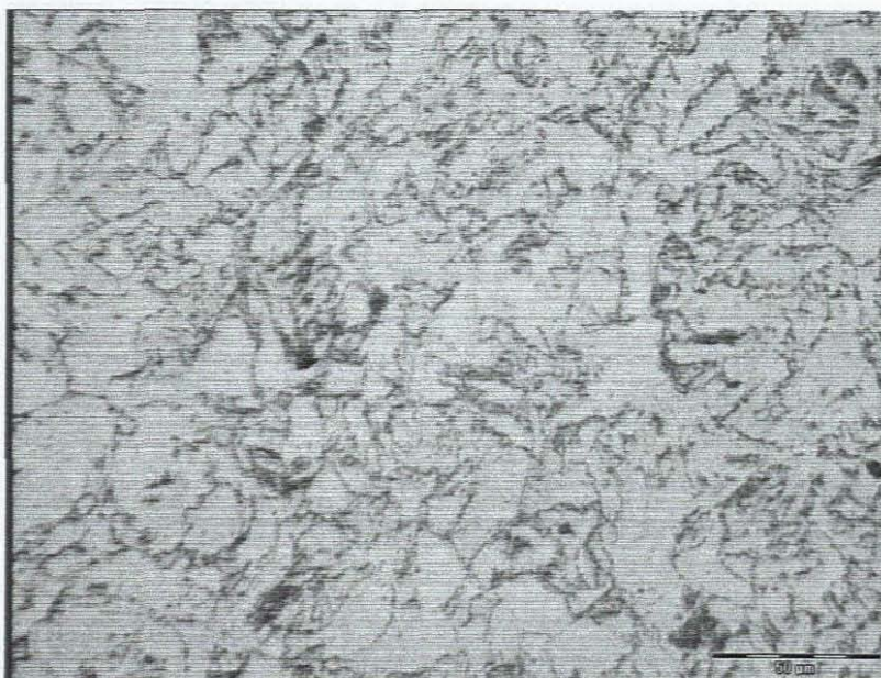
Figure 7.49: Microstructure of the HAZ specimen 4 depicts a structure of equiaxed ferrite grains with pearlite islands as seen at 50\mu\text{m} = 20\text{mm} \Rightarrow 400\times .
