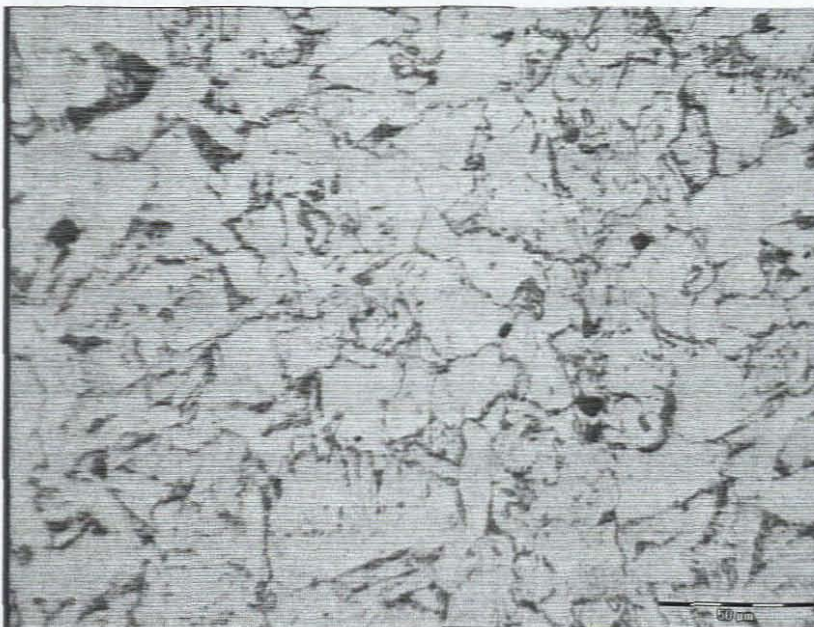
Figure 7.53: Microstructure of the HAZ specimen 5 depicts a structure of equiaxed ferrite grains with pearlite islands as seen at 50\mu\text{m} = 20\text{mm} \Rightarrow 400\times .
