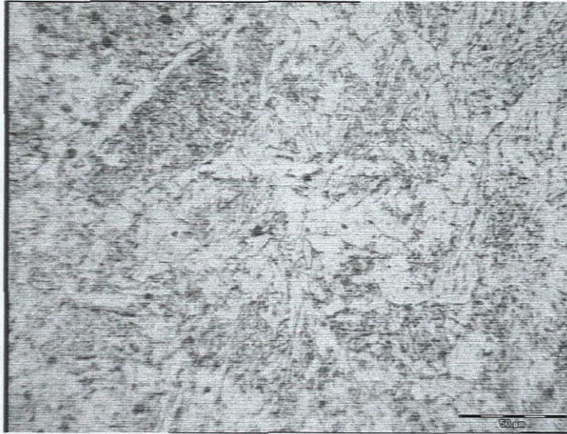
Figure 7.46: Microstructure of the weld specimen 3 depicts a structure of acicular ferrite with pearlite as seen at 50\mu\text{m} = 20\text{mm} \Rightarrow 400\text{x} .
