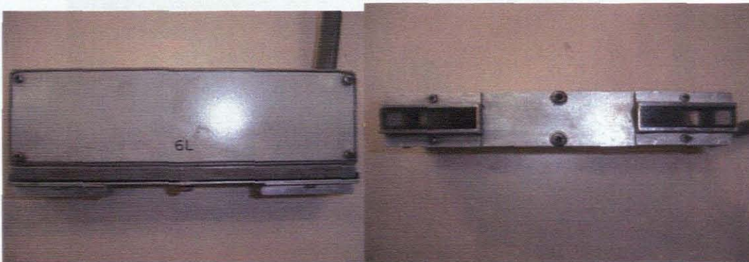
Figure 7.7: The 6L150 probe head used to measure subsurface stress.
