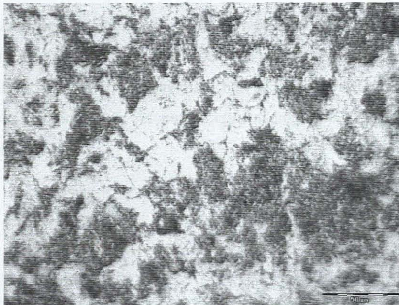
Figure 7.69: Microstructure of the HAZ specimen 5 depicts a structure of ferrite & pearlite as seen at 50\mu\text{m} = 20\text{mm} \Rightarrow 400\times .
