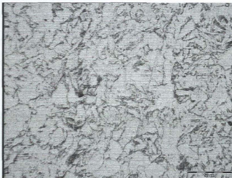
Figure 7.48: Microstructure of the plate specimen 4 depicts a structure of equiaxed ferrite grains with pearlite islands as seen at 50\mu\text{m} = 20\text{mm} \Rightarrow 400\times .
