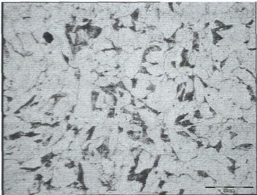
Figure 7.44: Microstructure of the plate specimen 3 depicts a structure of equiaxed ferrite grains with pearlite islands as seen at 50μm = 20mm ⇒ 400x.
