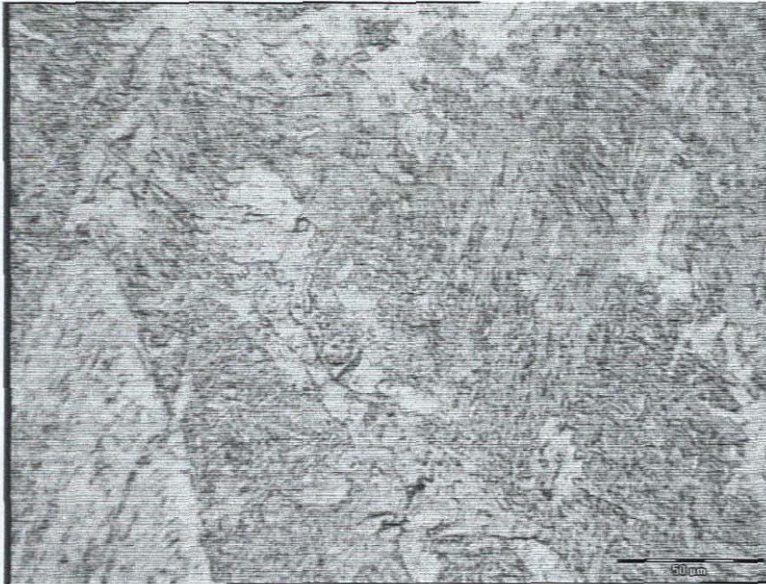
Figure 7.42: Microstructure of the weld specimen 2 depicts a structure of acicular ferrite (Widmanstätten structure) with pearlite as seen at 50\mu\text{m} = 20\text{mm} \Rightarrow 400\text{x} .
