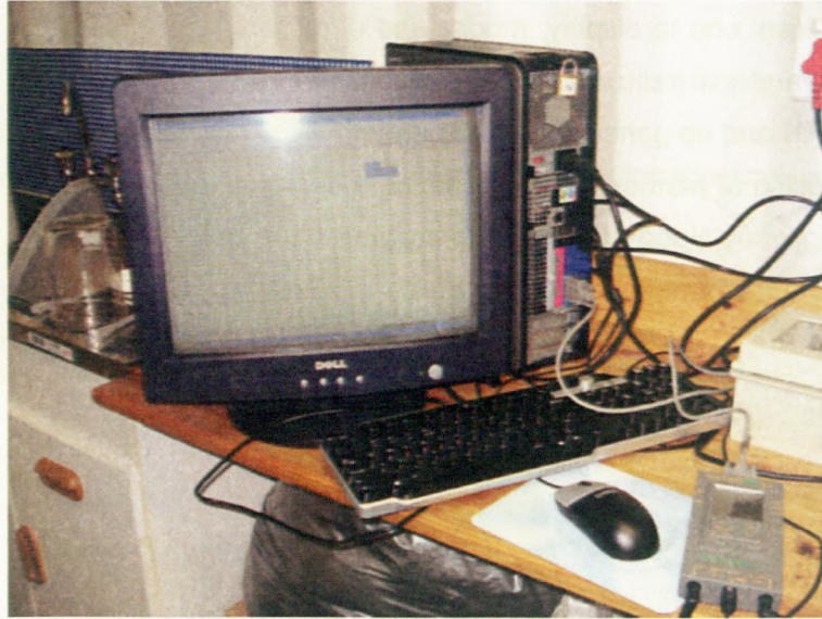
Figure 3.7: Connection of power and harmonic analyser to RS232 serial port of PC
