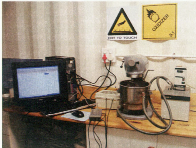
Figure 3.5: Modifications of Hobart N50 and Haake system
