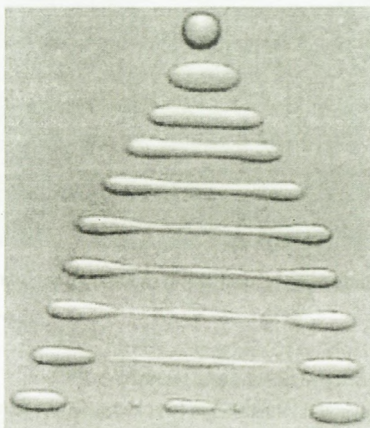
Figure 2.16: Necking mechanism (Adapted from Changzhi and Liejin, 2007)
