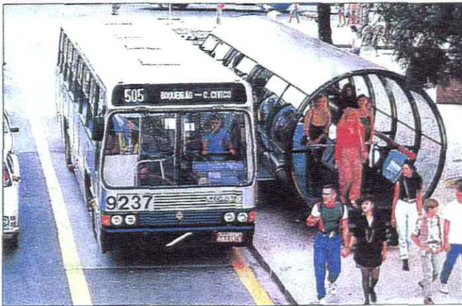
Figure 5.11 Curitiba has established an efficient network of buses with sheltered bus stops. For speeding up the service, ticketing takes place at the entrance to the bus stop (Source: International Union of Public Transport , 1996: 10).
