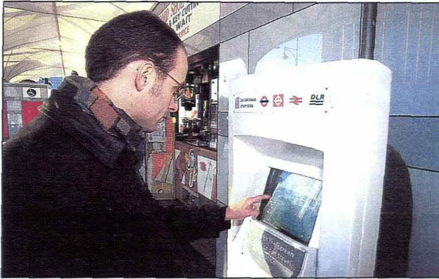
Figure 5.2 A touch-screen passenger-access terminal where information can be tailored to specific requirements (Source: Transport for London Integration Department, 2001: 27 ).
